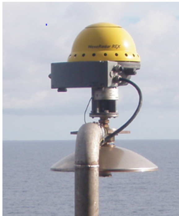
Plate 1: WaveRadar REX mounted on a South China Sea platform.
